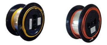
Dummy fiber is designed to be used in conjunction with an OTDR to measure complete link loss of a fiber. They are also known as pulse suppressor cables, launch cords, launch leads, receive cables or fiber rings. An OTDR dummy fiber, which connects the OTDR to the link-under-test, discloses the insertion loss and reflectance of the nearend connection. A fiber ring serves as both a launch cable and a receive cable.
